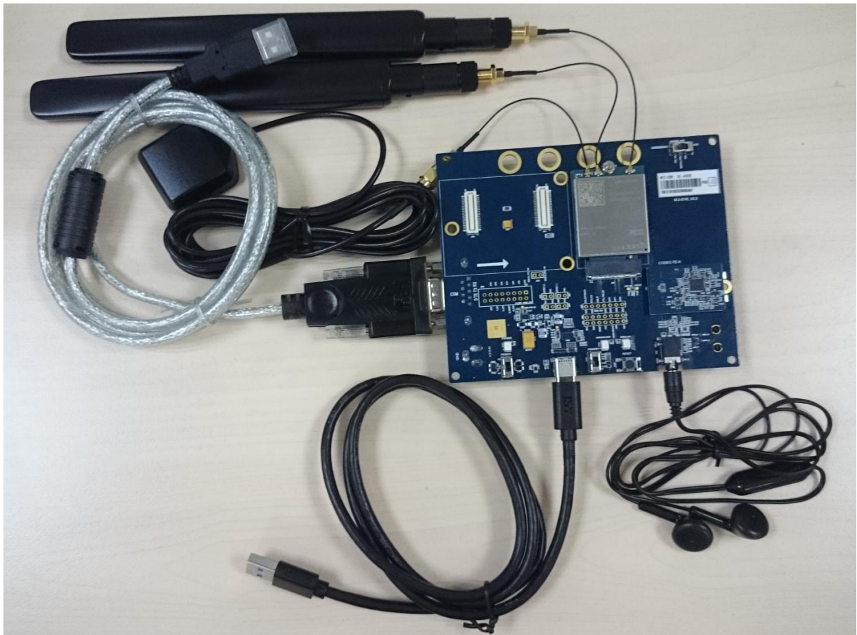
Figure 5: M.2 EVB Kit Accessories Assembly
