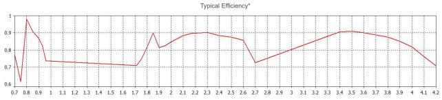
\*Typical efficiency simulated in CST Microwave Studio on 400x400mm (1.3' x1.3') ground plane excluding cable loss
