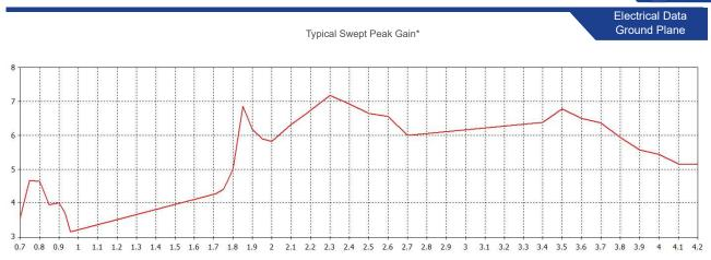
\*Swept peak gain simulated in CST Microwave Studio on 400x400mm (1.3' x1.3') ground plane excluding cable loss
