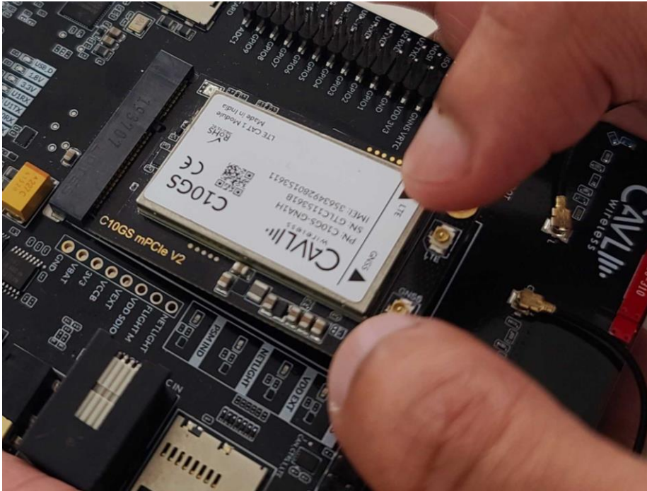
Figure 5 Aligning the 80-Pin Connector and its slot
