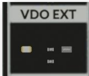
Figure 35 VDD_EXT voltage indicator
