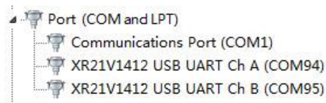
Figure 5: UART Ports Displayed on PC
