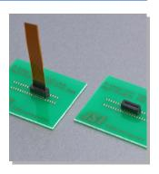
This is low profile 0.4mm pitch Non-ZIF top entry type connector with a mounting height of 2.5mm.
