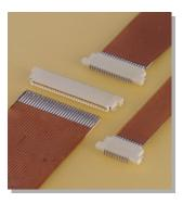
The large miniaturization at pitch direction and depth direction and low-profile as 1.2mm mounting height are realized. FH connector is miniaturized and space saving Non-ZIF type connector for FPC.
