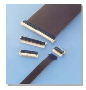
This connector for the 0.3mm thickness FPC with a mounting height of 1.3mm. FPC with protrusion prevents incomplete insertion and mis-insertion, so that it provides reliable connection.
