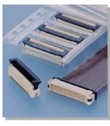
Vertical 0.3mm pitch ZIF type connector. This connector was mainly developed to connect FPC and subminiature digital products such as DVC, DSC, PDAs and so on.
