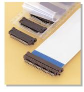
\*Connection can be made simply by inserting the leads into the connector and pressing the slider. Once the leads are inserted, they are held by the 4-side guides located inside the slider so that they will not dislocate or come off.
