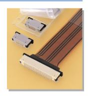
This is a 0.5 mm pitch, compact FFC/FPC connector with a mounting height of 2 mm. It features Zero Insertion Force (ZIF) connection, which is effective in improving wear resistance and insertion/withdrawal life. Both normal (upper contact type) and reverse (bottom contact type) connection types are available, contributing to greater flexibility in the design process.
