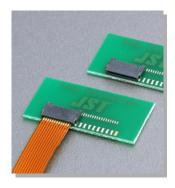
This FHA connector is a renewal product of current FHJ connector. This is Non-ZIF type connector for the 0.3mm thickness FPC with a mounting height of 1.1mm, small and space saving type.
