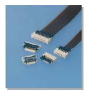
FHS connector is a space-saving type connector for FPC with 3.1mm depth, though it is low profile of 0.9mm mounting height. 0.2mm thick standard FPC.
