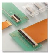
This is connector with the double-sided contact for FPC. As FPC with protrusions is used for this FHH connector, prevention of incomplete insertion and mis-insertion are realized and connection reliability is improved.
