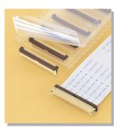
The FAZ connector is SMT type for PC board connector, which is a Zero Insertion Force (ZIF) type for FFC connection with a lead pitch 1.0 mm.
