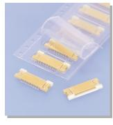
This is a 0.5 mm pitch FPC connector with a mounting height of 1.2 mm, compatible with standard FPCs with a terminal (lead) thickness of 0.3 mm. This connector features a Zero Insertion Force (ZIF) connection to effectively extend the lifespan of FPCs by reducing wear during mating and unmating.
