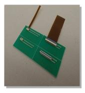
This ZIF type 'flip lock' FPC connector achieves a low-profile feature of a 0.9mm mounting height despite the thickness of the FPC being 0.3mm.
