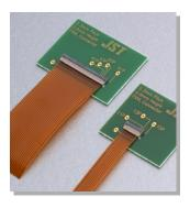
This FXVL connector is a space saving and low profile connector for FPC demanded from the market, and realizes 0.3mm pitch connector with a mounting height of 0.9mm and depth of 2.68mm.
