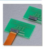
This is a 0.4 mm pitch, compact Non-ZIF type connector with a mounting height of 1.0 mm and a depth of 3.0 mm.
