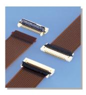
In addition to achieving space saving and low-profile features demanded by the market, this connector also realizes superb operability by adopting a FPC with protrusion. The use of the FPC provides secure and foolproof mating at the customers' production site.
