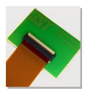
This is low profile and space saving type connector for FPC with 0.2 mm pitch, 0.95 mm height, and 3.0 mm depth. Back flip type of double-sided contact improves the freedom for routing of FPC.
