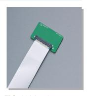
This is 0.5mm pitch connector for FPC which has the exclusive GND contact and enables high-speed transmission with connecting to the impedance controlled FPC. Adopting the auto lock mechanism that makes lock by performing the one action of snap-in-work, the workability improvement is realized.
