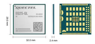
Quectel EG25-GL is an LTE Cat 4 module optimized specially for M2M and IoT applications. Adopting the 3GPP Rel-11 LTE technology, it delivers maximum data rates up to 150 Mbps downlink and 50 Mbps uplink. Designed in the compact and unified form factor, EG25-GL is compatible with Quectel UMTS/HSPA+ UC200A-GL module and multi-mode LTE Standard EC2x series (EC25 series, EC21 series and EC20-CE)/EC200A series/EG21-G/EG25-G modules, which allow for flexible migration among them in design and use.
